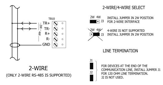
Install the following jumpers for the RS-485 interface according to the selected configuration:
