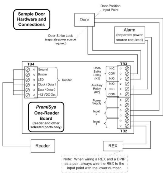
Connecting Inputs and Relays on the One-Reader Board
