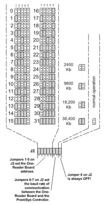
In the drawing above, an address of "0" is set on the One-Reader Board by removing the jumpers from positions 1-5, on jumper J2. An address of "23" is set by removing only the jumper in position 4 and installing the jumpers on positions 1-3 and 5.
