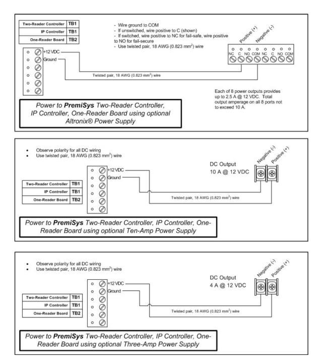
CAUTION! The processor in this component is intended for use only in a Class 2, low-voltage circuit!
