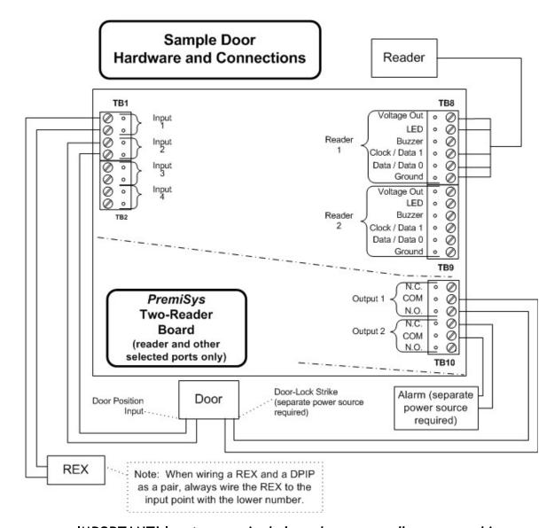
IMPORTANT! Inputs on a single board are normally processed in ascending numeric sequence when they change state simultaneously or nearly simultaneously. Consequently, if wiring a REX input point and a door-position input point in a pair, make sure that the doorposition input point has a higher input number than the REX point paired with it.
