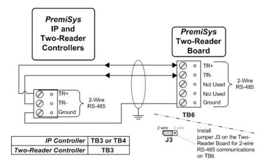
MPORTANT! Install Jumper J3 exactly as illustrated in the diagram above! Four-wire RS-485 cannot be used!
