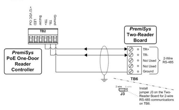
IMPORTANT! Install Jumper J3 exactly as illustrated in the diagram above! Four-wire RS-485 cannot be used!
