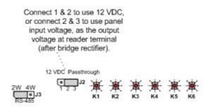
Refer to the documentation enclosed with individual readers to determine if the readers must have their own separate power source and not be powered from the Two-Reader Board.
