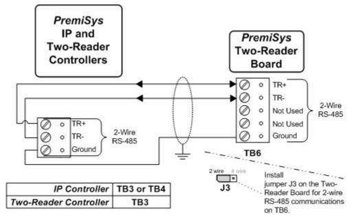
On the PremiSys™ IP Controller, terminal blocks TB3 (Port 2) and TB4 (Port 3) are used for connection to I/O boards.
