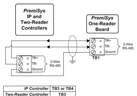
On the PremiSys™ IP Controller, terminal blocks TB3 (Port 2) and TB4 (Port 3) are used for connection to I/O boards.
