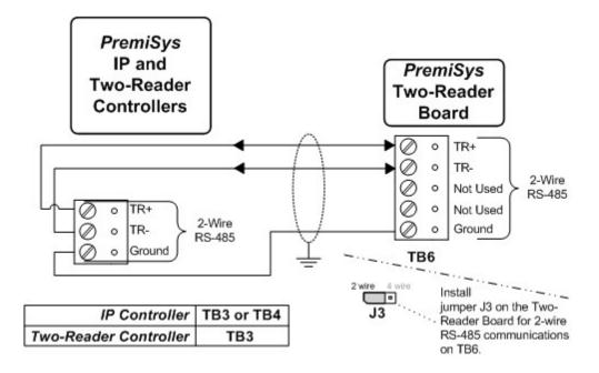
Port 2 on the Two-Reader Controller – RS-485 to TB 6 on the Two-Reader board Two-wire RS-485 2,400-38,400 bps, asynchronous Twisted pairs, 22 AWG (0.325 mm2), with overall shield
