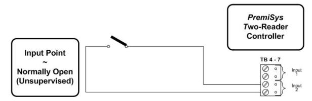
Wiring a Two-Reader Controller to the PoE One-Door Reader Board
