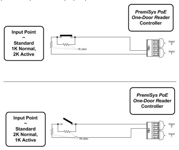
Wiring Unsupervised Input Points on the PoE One-Door Reader Controller
