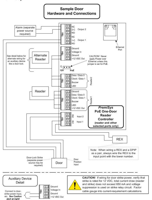
Wiring a PoE One-Door Reader Controller to Door Strike and Magnetic Lock
