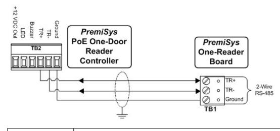
TB2 on the PoE One-Door Reader Controller – RS-485 to TB 1 on the One-Reader board Two-wire RS-485
