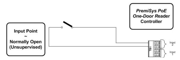
Wiring a PoE One-Door Reader Controller to the PoE One-Door Reader Board
